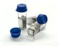
Cuvettes for in-vitro electroporation. These are plastic with aluminium electrodes and a blue lid. They hold a maximum of 400  $\mu$ l.
